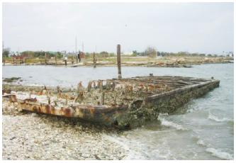
Corroded steel barge on Lavaca Bay Shoreline in Calhoun County.
