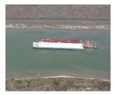
Tugboat pushing barge to efficiently transport petrochemicals along the GIWW.
