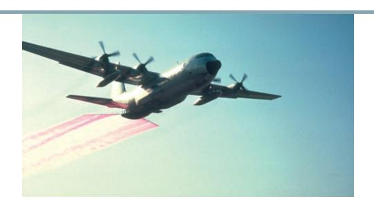
Dispersant application from a C-130 Hercules using an Aerial Dispersant Deployment System (ADDS). The dispersant has been dyed red for experimental purposes.
