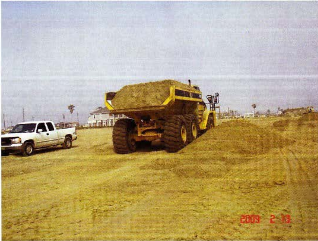
Figure 11. Heavy equipment used to transport clean sand used in renourishing Bolivar Peninsula and Galveston Island beaches.
