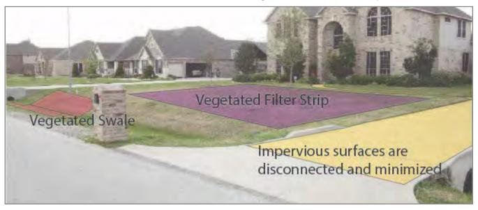
**Figure 4-2:** Medium density neighborhood uses vegetated swales for stormwater conveyance. These swales also provide water quality benefits.
