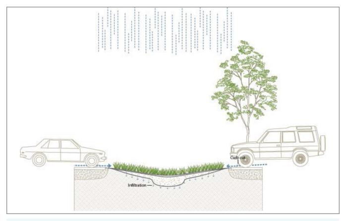
**Figure 5-2:** Swale in parking lot area. (Showing the use of short grasses, low slopes, curb cuts from parking area and some infiltration.
