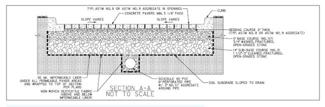
Figure 5-6: Representative cross-section of porous pavement.
