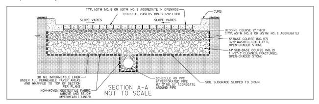
**Figure 5-6:** Representative cross-section of porous pavement.
