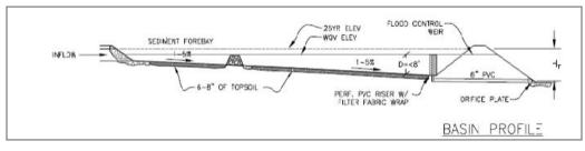
Figure 5-10: Schematic of an Enhanced Extended Detention Basin
