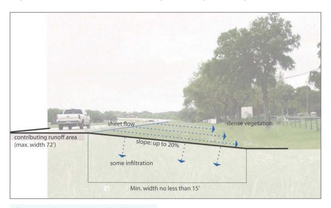
**Figure 5-3:** Filter strip along side of highway.
