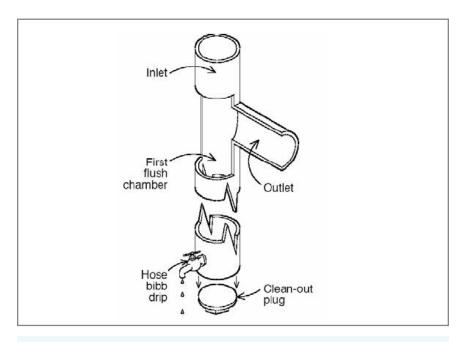
Figure 5-24: Standpipe first flush diverter. The recommended diversion of first flush ranges from one to two gallons of first-flush diversion for each 100 square feet of collection area. (TWDB, 2005)
