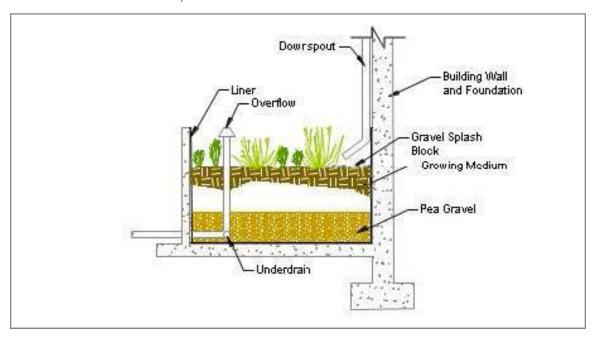
Figure 5-19: Stormwater Planter Box (Harris County LID Manual)
