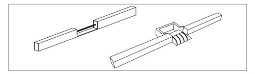
**Figure 5-17:** Curb cuts with optional sediment/trash screens.
