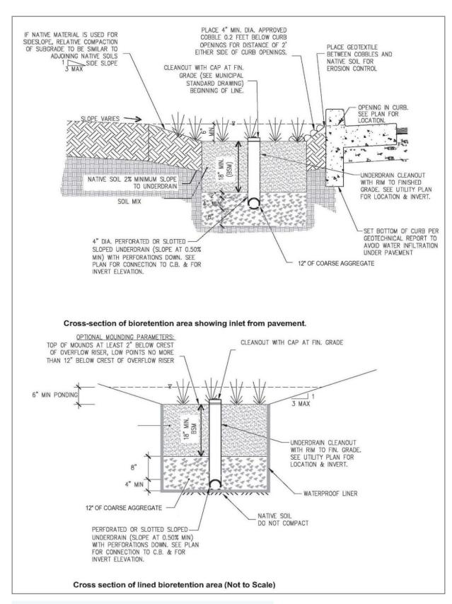
**Figure 5-13:** Schematic diagram of a bioretention system.
