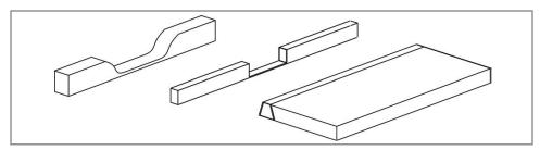
**Figure 5-16:** Curb cut options: smooth cut, hard cut and flush curb.
