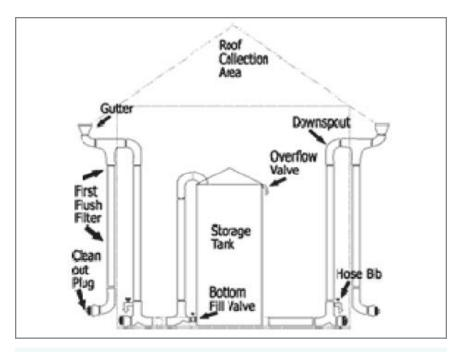
Figure 5-23: Complex water harvesting system (with roof catchment, gutter, downspout and storage tank. City of Austin Energy's Green Building Fact Sheet, 1995).
