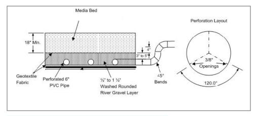
**Figure 5-15:** Illustration of optional outlet design.
