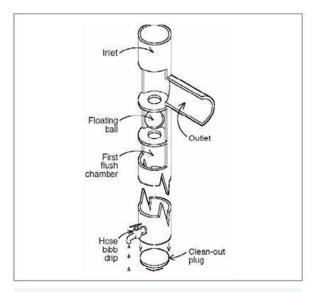
**Figure 5-25:** Standpipe with ball valve. The standpipe with ball valve is a variation of the standpipe filter. As the chamber fills, the ball floats up and seals on the seat, trapping first-flush water and routing the balance of the water to the tank. (TWDB, 2005)
