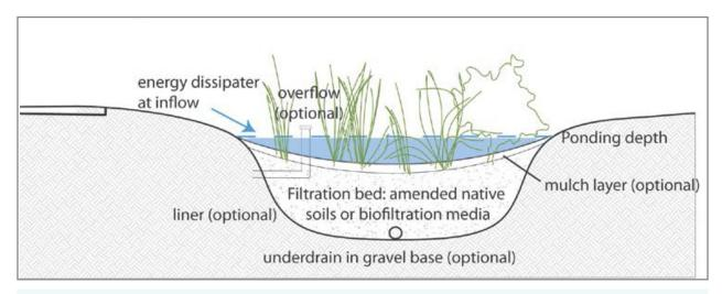
**Figure 5-11:** A diagram of the basic rain garden / bioretention system components including optional components.
