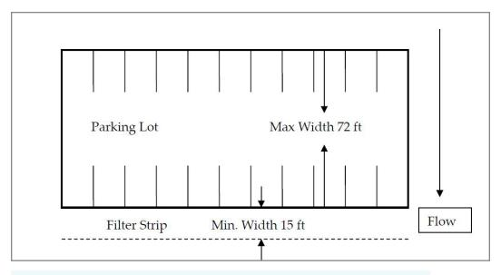
**Figure 5-4:** Example configuration of filter strip adjacent to a parking lot.
