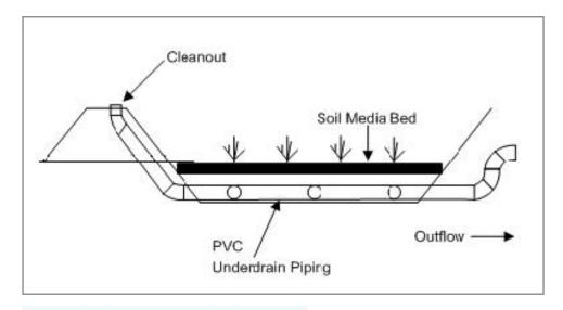
**Figure 5-14:** Detail of cleanout location.
