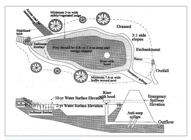
Figure 5-9: Schematic of a wet basin.
