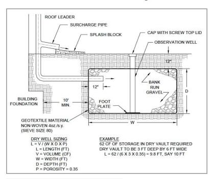
Figure 5-27: Schematic of Dry Well
