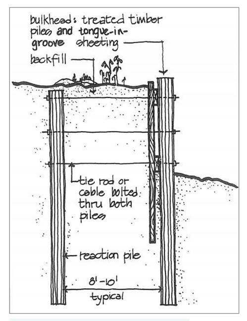
Figure 6-20: Schematic Bulkhead Example (Source: EPA)
