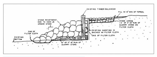
Figure 6-21: Schematic Toe Protection (Source: EPA)
