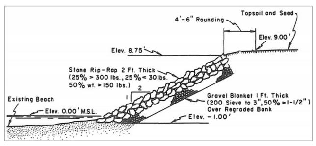
Figure 6-22: Rock Rip Rap Schematic Cross Section (Source: EPA)
