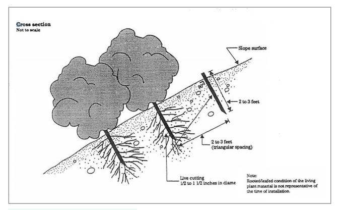
Figure 6-16: Live Staking (Source: EPA)
