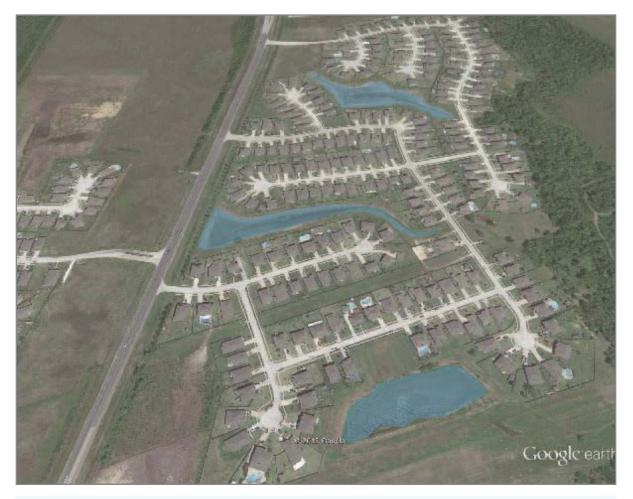
**Figure 6-5:** Layout of a high-density single-family residential development. Includes three detention ponds.
