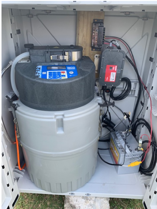
Figure 6. ISCO 6712 sampler, modem, power supply and array connections inside the sampling boxes.
