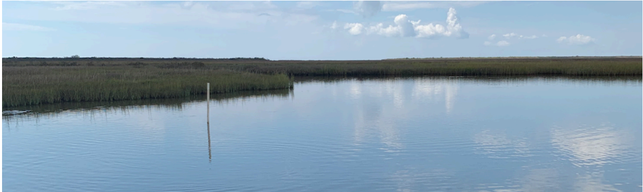
Fig. 6. The CTDs were installed inside of PVC pipes and placed into water bodies or channels.
