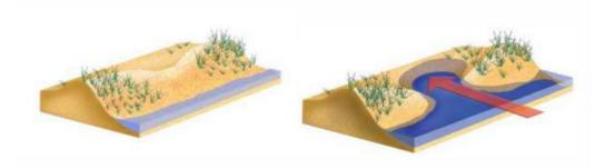
Figure 7: Washover Damage to the Dune System
