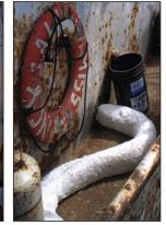
Place spare pads / sorbent material around fuel fill to capture any fuel spilled on deck.
