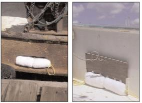
Insert sorbent pillows tightly into freeing ports -No gaps! Secure pillows in place with wooden scupper boards.
