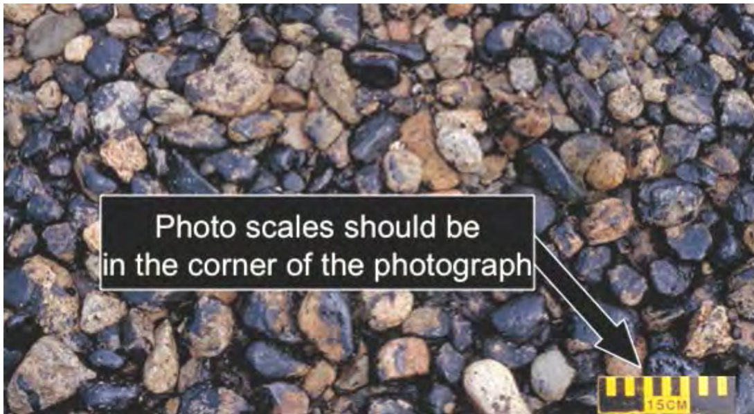
Where to put the photo scale when taking a photograph of the ground surface.
