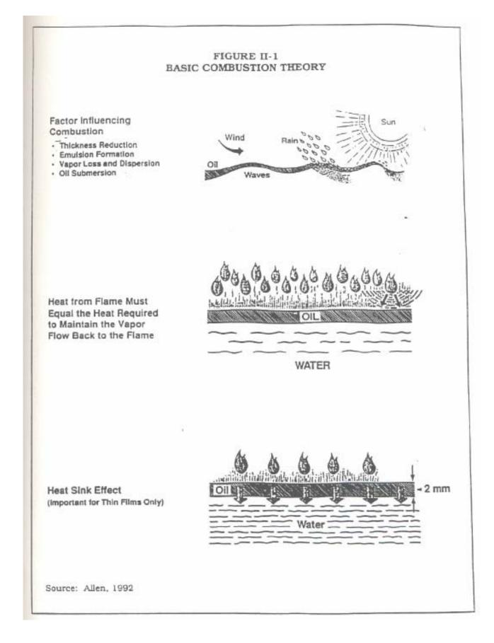
As shown in Figure II-1, the heat radiated back from the flame (typically only 2% to 3% of the heat generated) must equal or exceed the heat required to maintain the vapor flow from the oil back to the flame. If the oil is too thin (usually about 1 to 2 millimeters for fresh oil), the "heat sink" effect of the water will be sufficient to cool the oil to the point where vapor production will be too low to sustain the fire.
