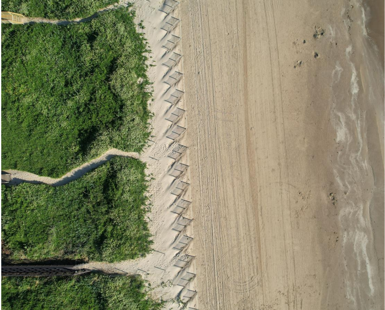
Figure 1. Project layout showing fencing orientation with native dune vegetation planting behind the sand fencing.
