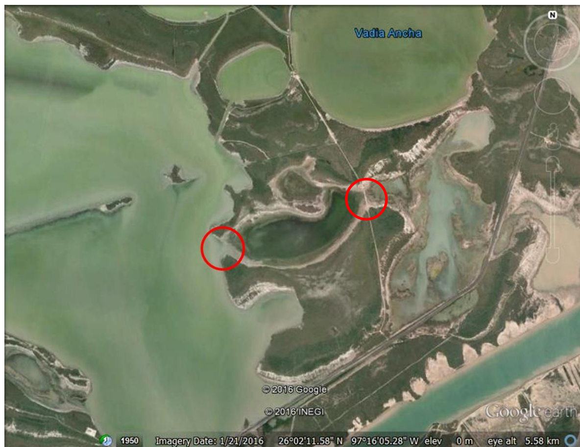
Figure 12. Sand Bar(s) to be Removed to Open Paso Corvinas to Tidal Exchange 8
