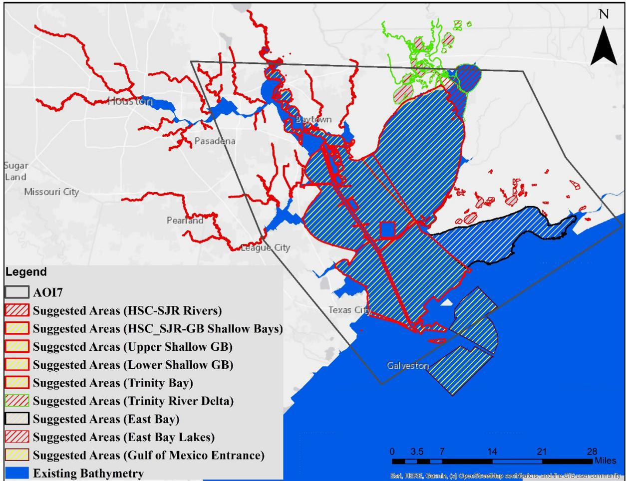
Figure 24. Existing bathymetry and the suggested area to acquire bathymetric data based on data availability of year of last acquisition for AOI 7. Please also refer to AOI 4, 11, and 13 for more information on some of the suggested areas shown here and not listed under AOI 7. Different hatched colors are not clearly distinguishable in the figure to the number of active layers. All the GIS files can be found [here](#).
