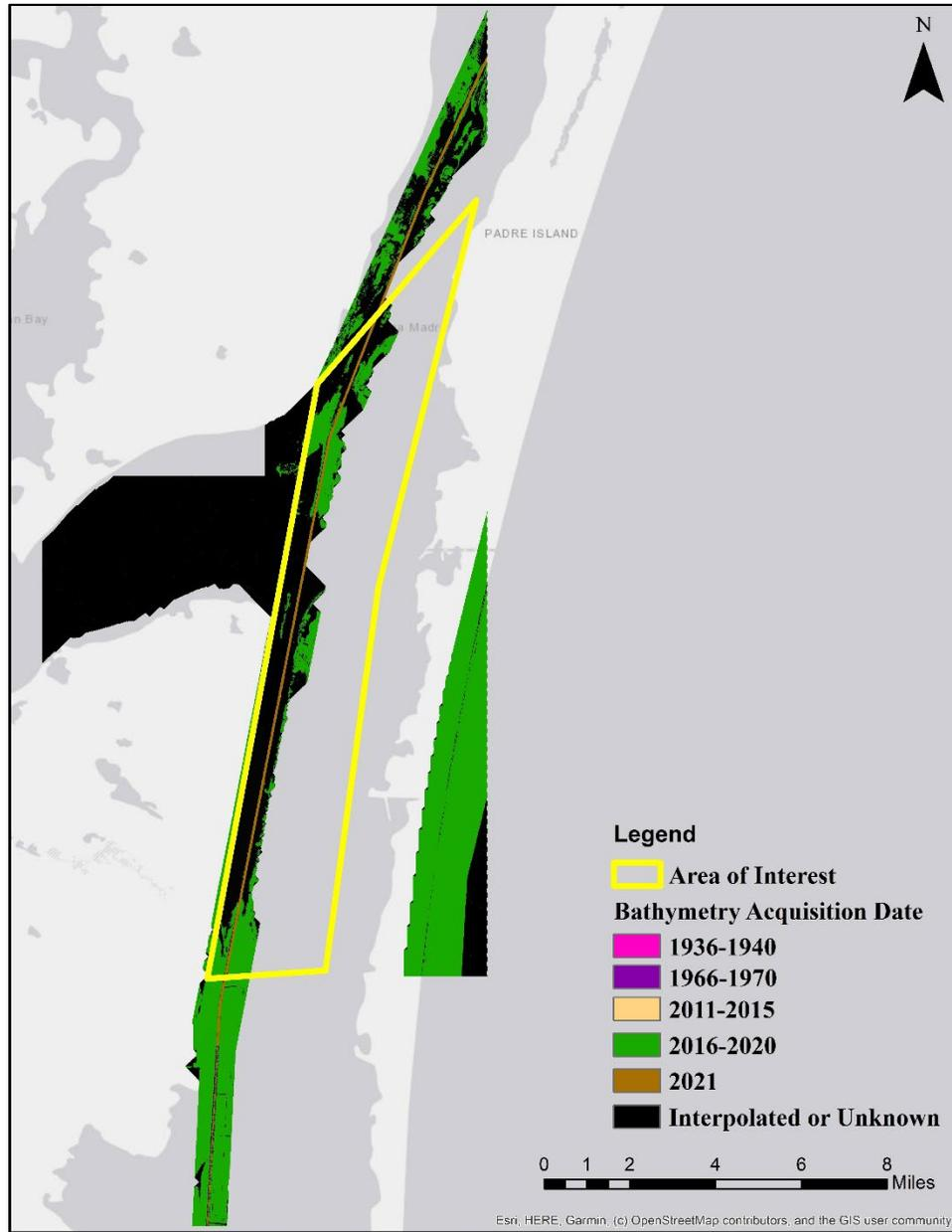
Figure 16. Latest bathymetry acquisition date for AOI 5 using the BlueTopo database.
