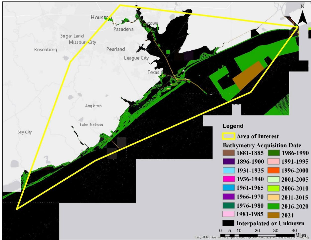
Figure 32. Latest bathymetry acquisition date for AOI 11.
