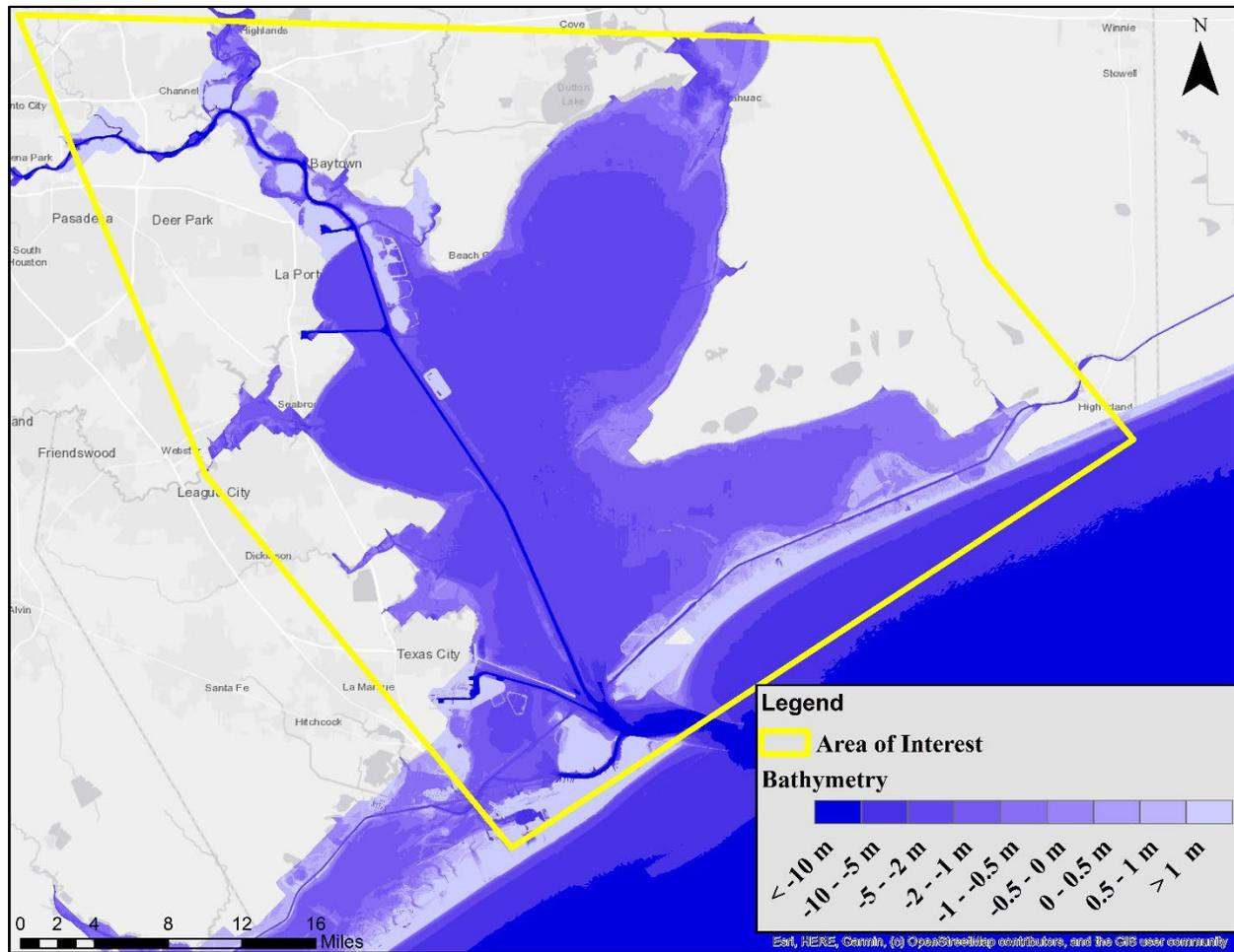
Figure 22. Bathymetry of AOI 7 using the BlueTopo and the TPWD databases.
