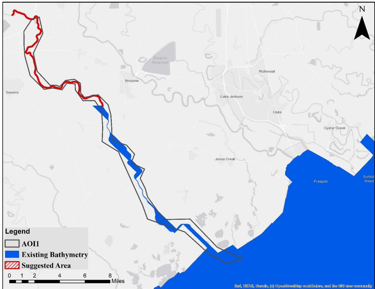
Figure 5. Existing bathymetry and the suggested area to acquire bathymetric data based on data availability of year of last acquisition for AOI1.
