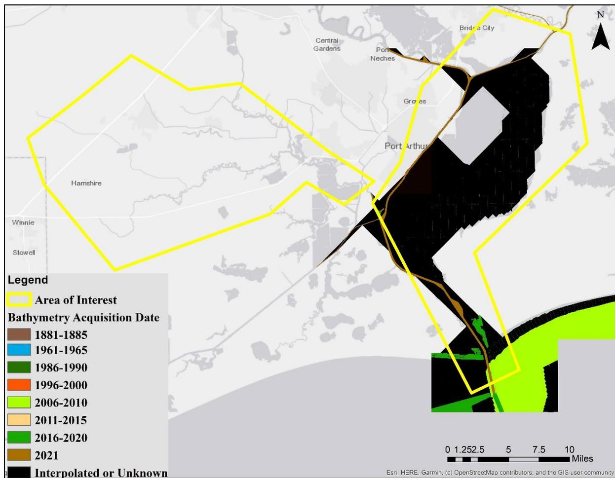
Figure 26. Latest bathymetry acquisition date for AOI 8 and 9 using the BlueTopo database.
