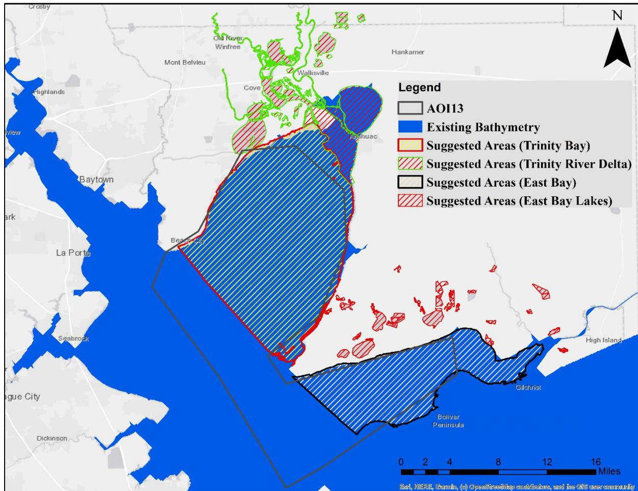
Figure 36. Existing bathymetry and the suggested area to acquire bathymetric data based on data availability of year of last acquisition for AOI 13. Please also refer to AOI 4, 7, and 11 for more information on some of the suggested areas shown here and not listed under AOI 13. Different hatched colors are not clearly distinguishable in the figure due to the number of active layers. All the GIS files can be found [here](#).
