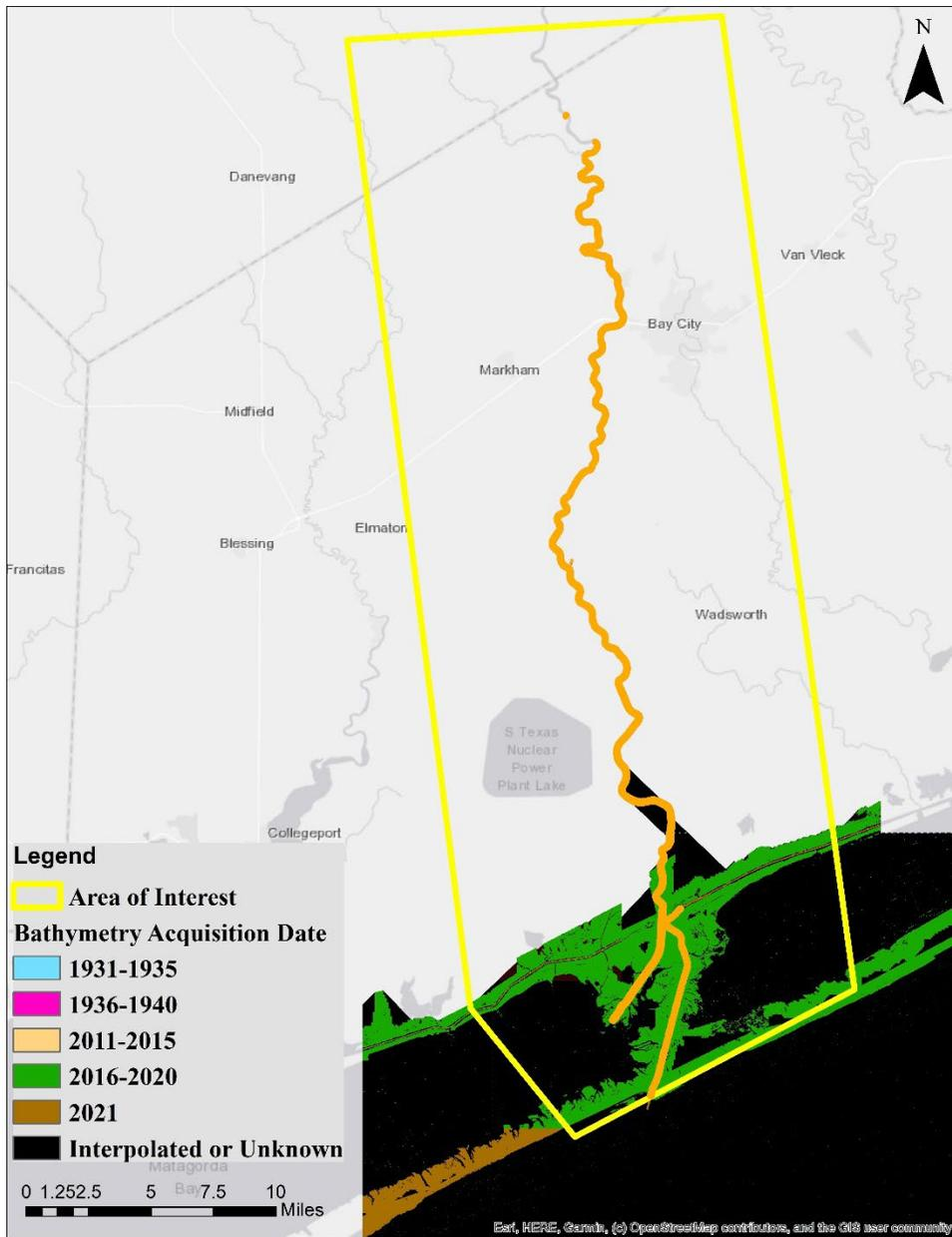
Figure 29. Latest bathymetry acquisition date for AOI 10 using the BlueTopo database.
