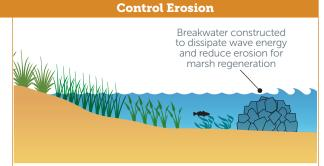
Breakwaters can prevent erosion from the seaward side of estuaries by reducing wave action along a shoreline. They can be constructed of natural materials and aid in building up estuarine habitats.
